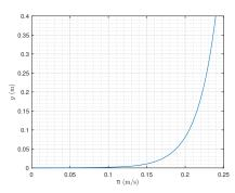
Example mean velocity distribution,  $\overline{u}$ , considering shear current theory with the van Driest solution
