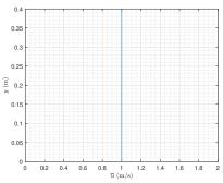
The potential current approach does not resolve different flow characteristics for the entire water depth as the theory assumes a fixed velocity for the entire flow section. As an example, if one wants to study the sediment motion which mobilizes from the bed and generally transports in the boundary layer (for the current it is the full water depth), the potential current theory results do not give realistic results.
