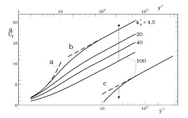
Example of van Driest velocity profiles for different values of roughness (Taken from [SF20], Figure 3.21 at page 101)
