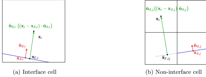
Figure 5.2: Illustration of how to compute the interface position using cell center, interface center and interface normal
