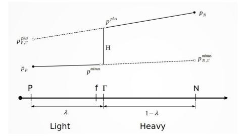
Figure 3.2: One-sided interpolation for a dry owner cell.
