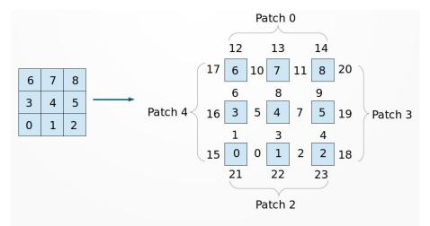
Figure 2.5: Example domain with 9 cells, 11 internal faces and 30 boundary faces. The top, bottom, left and right side of the domain is 4 patches, and each patch has 3 boundary faces. The remaining 18 boundary faces, not included in the illustration, are found on the back side and front side of the cells.
