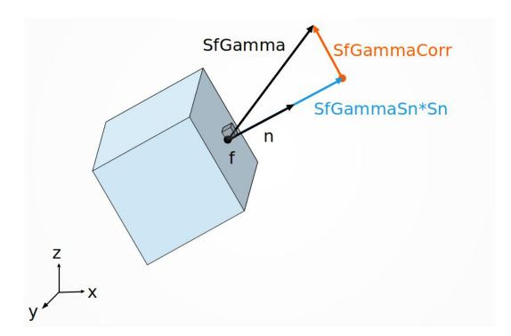
Figure 2.4: Illustration of mathematical operations performed when the diffusion coefficient is a tensor  $\gamma_f$ . The operations are performed in the function fvmLaplacian in gaussLaplacianScheme.C, Line: 167 - 174.
