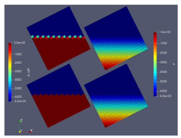
Figure 4.2 shows a visual comparison of the dynamic pressure distribution calculated with the two different schemes.
