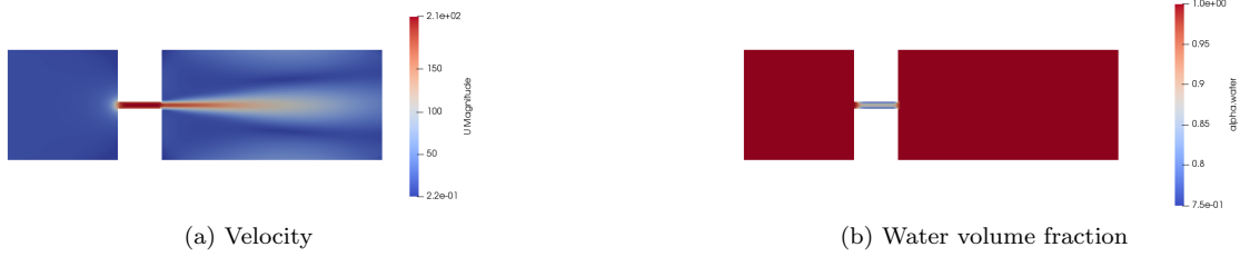
Figure 2.2: Last time step for throttle tutorial solved with interPhaseChangeFoam and Schnerr-Sauer cavitation model.
