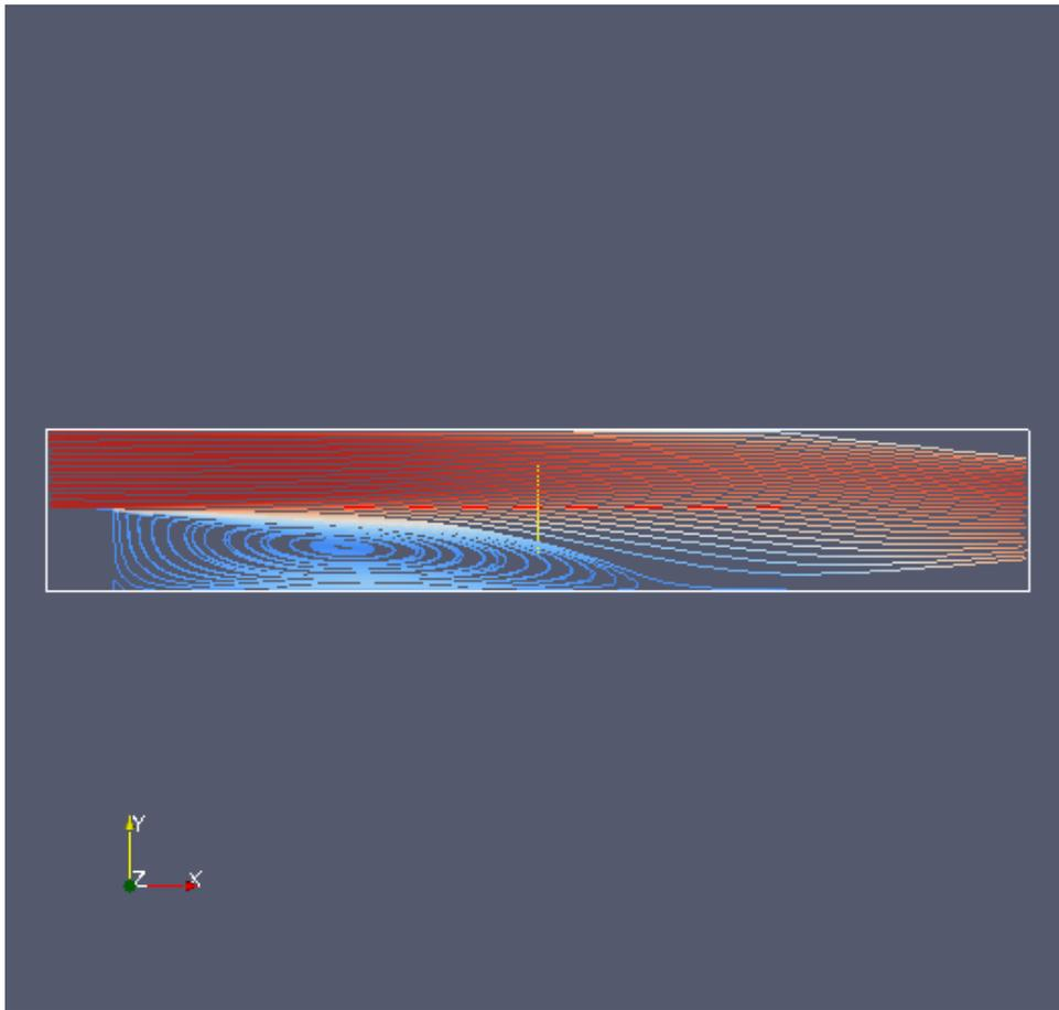
Pressure on streamlines, capturing the vortex behind the inlet wall.
