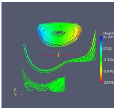
Three sets of streamlines, showing the main vortex, the field just above the corner box (it seems still to be some residual flow through the boundary), and the secondary vortices at the bottom, respectively.
