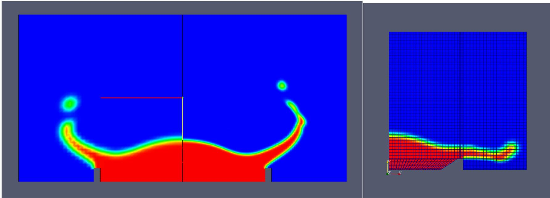
Both simulations in the same plot, having changed "Orientation" in the transformation box to 180 degrees around the y-axis. (For some reason, changing the x Scale to -1 produced a black box.) The variable plotted is "Gamma", i.e. the liquid content, showing a formation of a splat droplet, smaller and faster in the case of the finer mesh. Separate picture showing the modified simulation, with one point moved to the left to give the obstacle a different shape.
