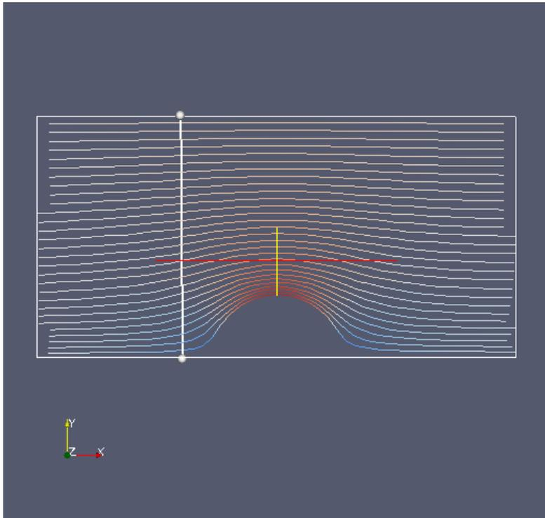
Streamlines on the cylinder. It was necessary to reduce the initial step length from 0.5 cell lengths to 0.1 cell lengths in order to avoid streamlines through the cylinder.
