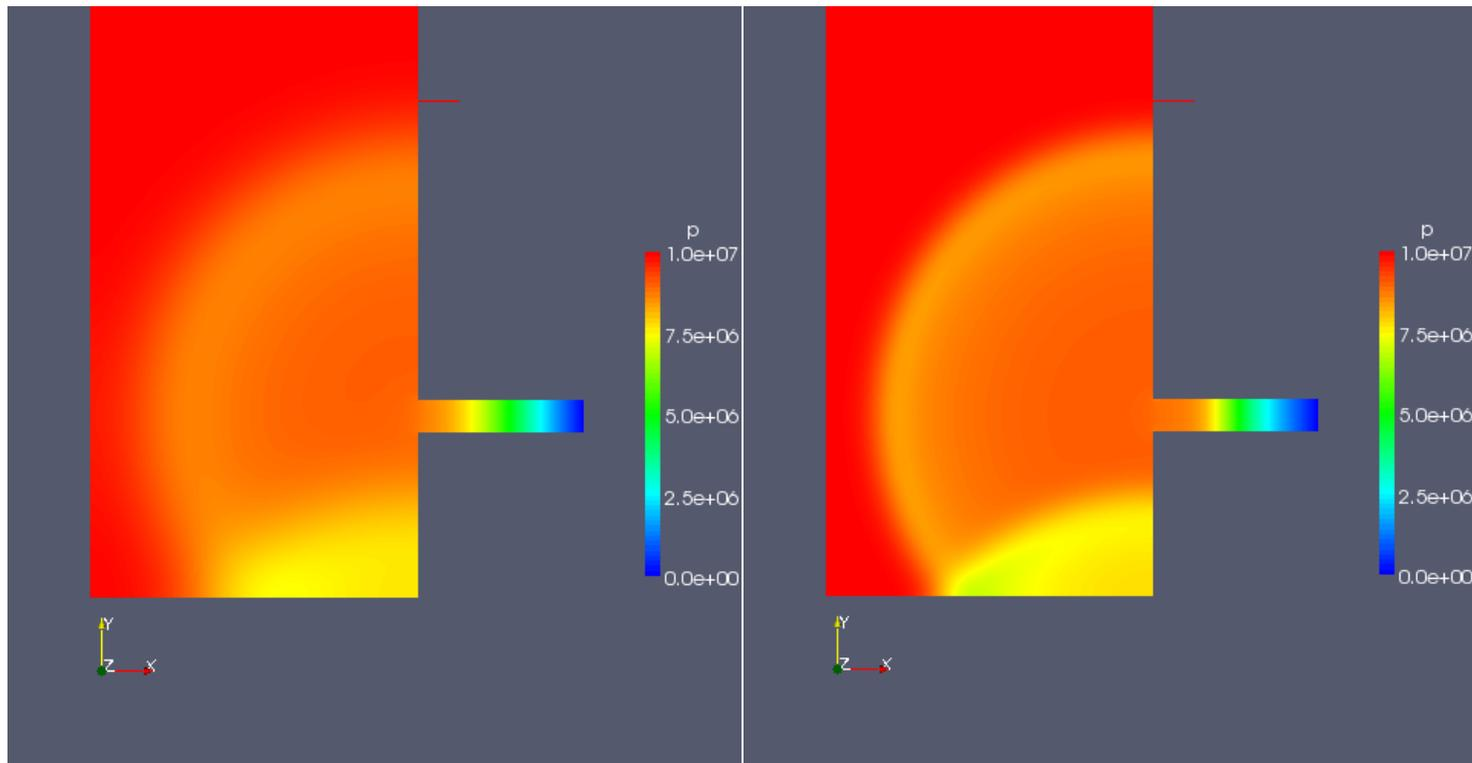
Pressure plots at the same time,  $70\mu\text{s}$  (step 9 and 45, respectively), showing the sharper pressure front in the finer mesh.
