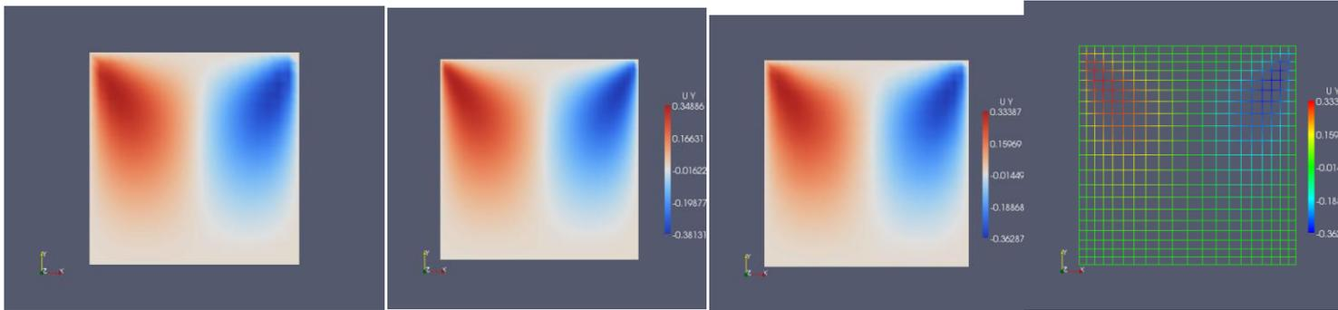
Velocity in the y-direction plotted for the three cases, not showing much of a difference. Wireframe plotted using "Use parallel projection" under "Render view options".
