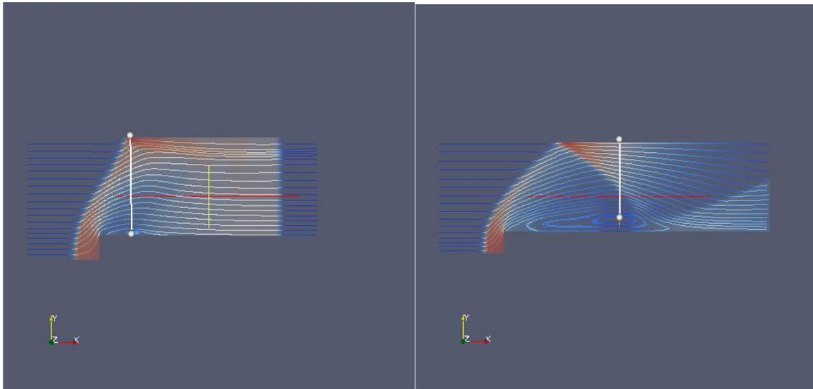
Pressure on streamlines again (I like that). The left picture is from very early in the simulation, just as the shockwave has hit the step, while the second is the stationary shockwave pattern, including a much more developed turbulence pattern. The line for streamlines is moved between pictures and plotted for reference. A start step of 0.1 cell lengths was used.
