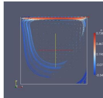
Pressure on streamlines, showing the small secondary vortex in the corner, caused by the High Reynolds number.
