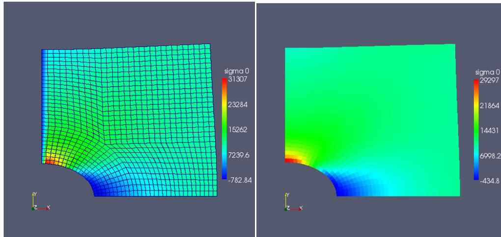
The extrapolation of stresses to the symmetry line  $x=0$  is not correct as seen in the left picture. Using element stresses, as in the right, shows that the calculation is correct, though.
