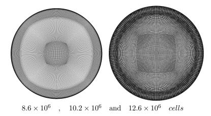
Two O-grids and three numerical schemes (first and linear order upwind) and linear limited (TVD) are examined.
