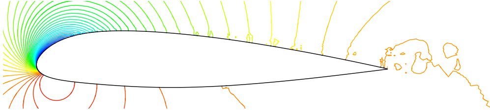
Figure 11: Instantaneous resolved pressure on the Chalmers mesh when wall functions are used (Comp. # 4).
