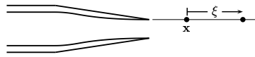
Figure 13. Two-point space-time correlations were evaluated in shear layer locations along the nozzle lip line, x . The spatial separation, \xi , is downstream in the axial direction.
