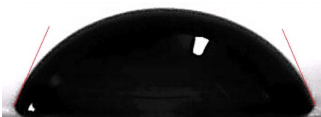
Figure 5.3: Measurement of the static contact angle
