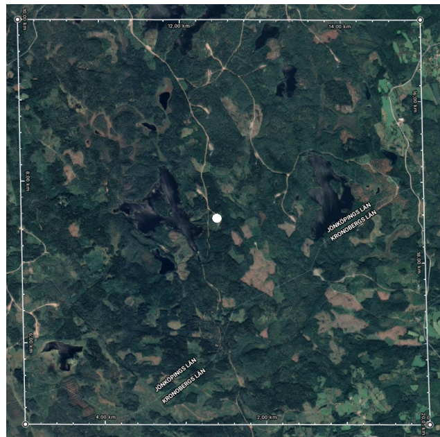
Figure 2. Satellite view of the simulated region with the location of the computational domain marked by a square. The location of the LiDAR in the middle marked by a white dot.
