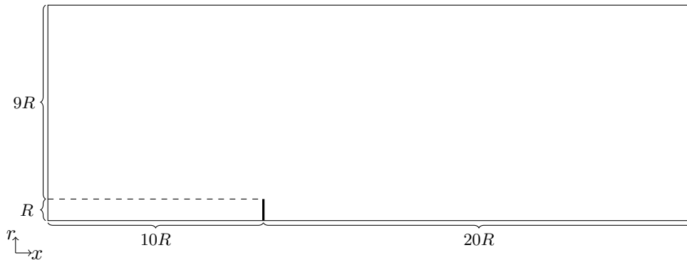
Figure 3.7: Axisymmetric computational domain in units rotor radii. The location of the wind turbine is seen as the thick line inside the computational domain.
