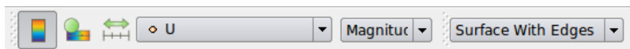
Figure 1.4: From the display options you can choose to view the velocity distribution U . In this case we have chosen to visualize the interpolated velocity distribution and also to show the mesh grid ( Surface With Edges ).
