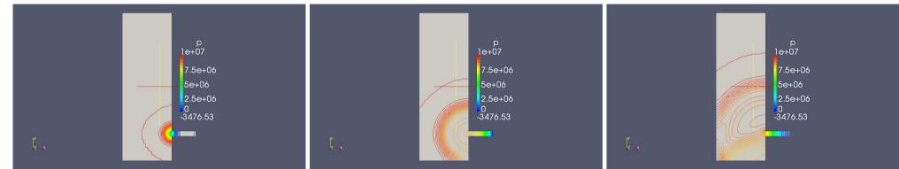
The three pictures above show contour snapshots of the pressure propagation after 40, 70 and 100 micro-seconds respectively. Contour plots are ahieved by simply using the "Contour" button on the menubar.
