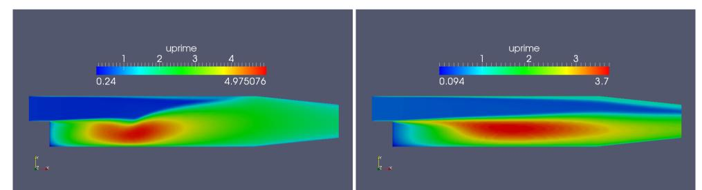
I increased the inlet velocity from 10m/s to 50m/s. In the controlDict I also changed the endTime to 240, the writePrecision to 2 and the writeInterval to 20. I then tried the utility *uprime* to compute and visualize the scalar field of u'. These scalar fields are shown above at two different time steps.
