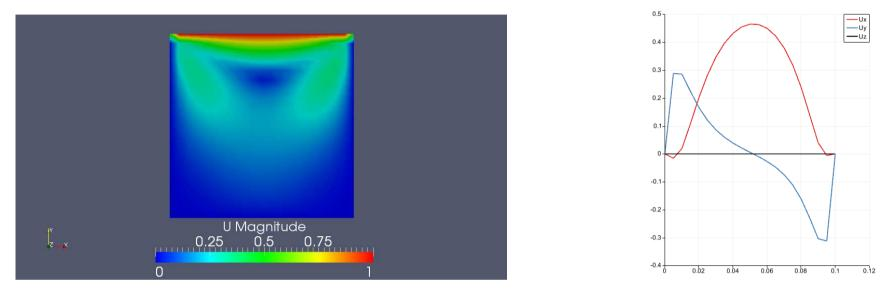
The left picture shows the interpolated velocity field. This can be visualized using "Display  $\rightarrow$  surface" and "color by  $\rightarrow \bullet$  U". Also, the color legend (Visualized by pressing "Toggle Color Legend Visibility") has been edited in "Edit Color Map" to "blue-to-red".
