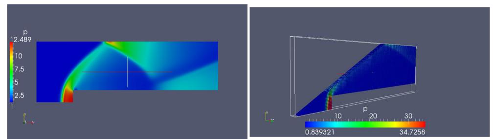
The left and right pictures show interpolated pressure distributions after 10 seconds with inlet velocity 3m/s and 5m/s respectively. The right picture features a "Clip" done along a shock wave and it is colored using the option "Surface With Edges" to show the mesh.
