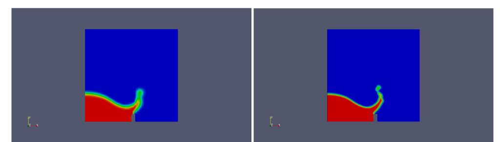
The left and right pictures show the "alpha1" distributions using a coarse and fine mesh respectively; both at t=0.2s. Snapshots from different timesteps can be achieved by clicking back and forth in the menubar between the loaded frames.
