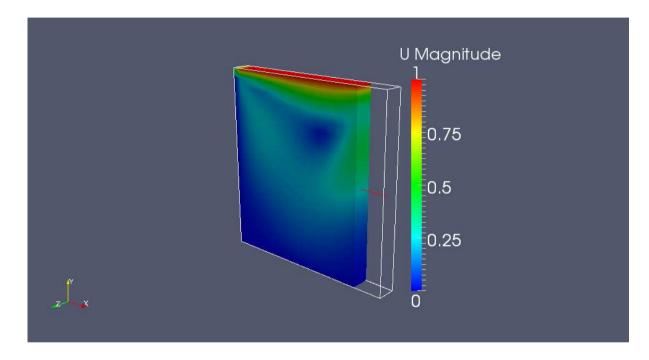
The picture above shows a clip done in the interpolated (i.e. colored by "• U") velocity field. A clip is done using the "Clip" button, and it can be positioned either by giving exact coordinates or by dragging it into place. Also, the entire domain is visualized by a frame using the "Outline" option.
