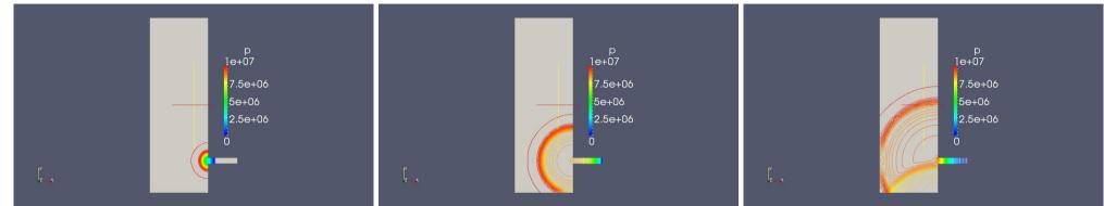
The three pictures above again show contour snapshots of the pressure propagation after 40, 70 and 100 micro-seconds respectively, but using a finer mesh than on previous slide.
