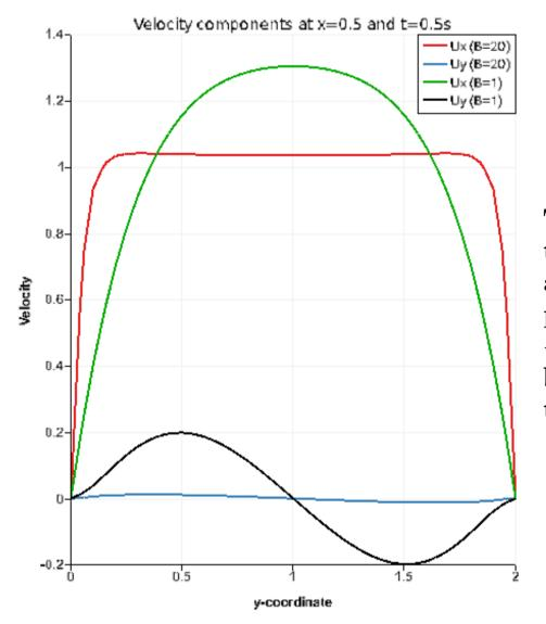
The picture to the left shows a comparison of the Ux and Uy velocity components for B=20 and B=1, at x=0.5 and t=0.5s, respectively. The plot is achieved using "Filters  $\rightarrow$  Data Analysis  $\rightarrow$  Plot Over Line", and the axes can be edited by clicking "Edit View Options" on the top of the plot window.
