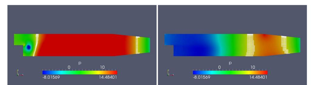
The left and right pictures show interpolated pressure distribution at 50 and 1000 iterations respectively. The mesh formations show areas where  $8 \le p \le 10$ . This effect is achieved using the "Threshold" option.
