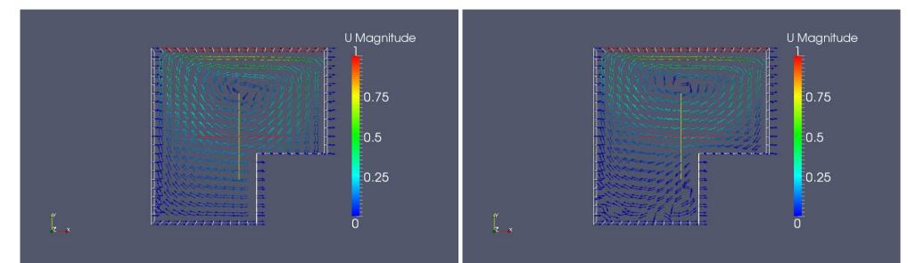
The left picture shows the velocity vector field after 0.5s and the right picture shows the velocity vector field after 0.6s. These are both visualized using "Glyph". The vectors are not scaled, but instead colored by "• U".
