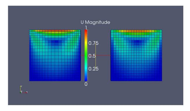
The picture shows the velocity fields for a graded and coarse mesh respectively. The vector fields have been positioned next to eachother using "Display  $\rightarrow$  Translate". The right picture shows a comparison of the Ux velocity component for a coarse and fine mesh respectively, between the points (0,0.09,0.005) and (0.1,0.09,0.005).
