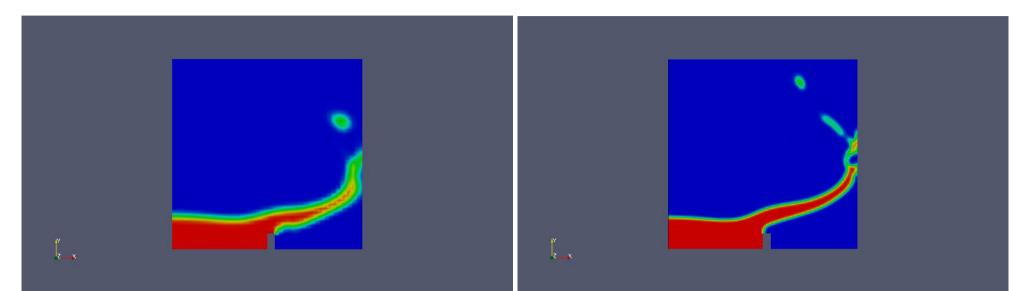
The left and right pictures again show the "alpha1" distributions using a coarse and fine mesh respectively; this time at t=0.35s. As can be seen in this and the preceding slide, the mesh resolution clearly influences the results.
