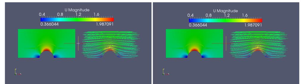
The left and right pictures show velocity fields and streamlines using nNonOrthCorr=0 and nNonOrthCorr=3 respectively. The velocity fields are visualized in the mid-plane of the domains using "Slice" from the menubar. The streamlines are visualized using the "Stream Tracer" option.
