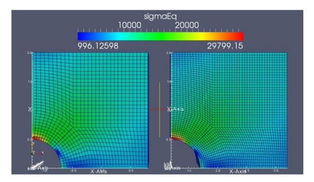
The picture above shows a comparison of the equivalent stress distribution between a coarse and a finer (x1.5 in x and y direction) mesh. They are colored using cell values (i.e. not interpolated). Also, the axes are visitalized via "Display  $\rightarrow$  Show cube axes".
