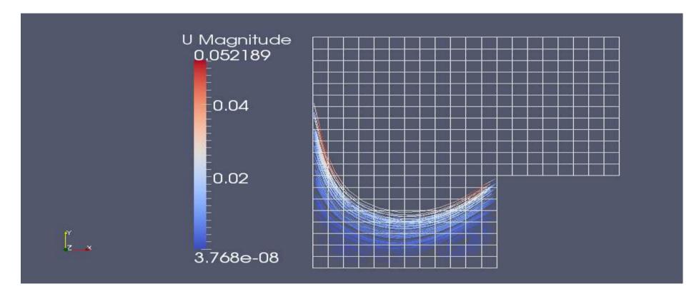
• Figure showing a "StreamTracer" placed at x = 0.03, y = 0.015, z = 0.005.
