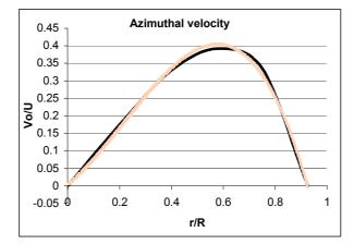
Figure a3: Azimuthal velocity profile as function of the radial coordinates r normalised on the rotor.
