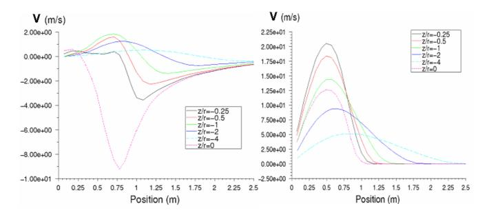
Figure a19: radial velocity profiles below the rotor as function of the radial coordinates r normalised
