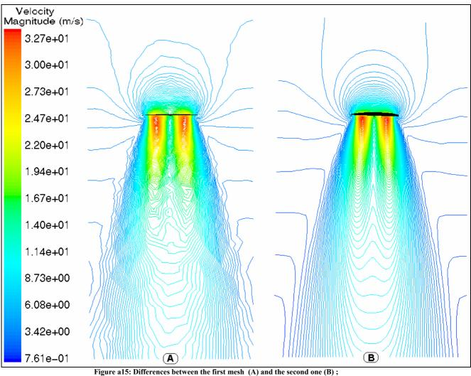
Visualization and Comparison of the contour of velocity magnitude on a plane
