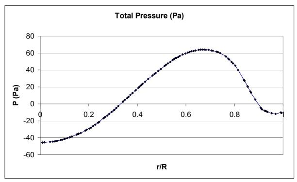
Figure a5: Example of Total pressure profile as function of the radial coordinates r normalised on the rotor calculated with Fluent.
