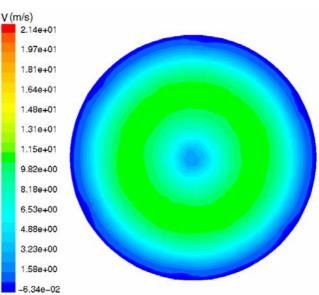
figure c8: Contour of tangential velocity on the rotor
