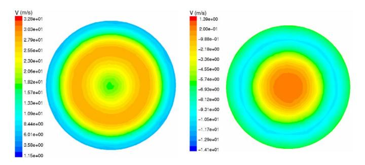
figure c5: Contour of velocity magnitude on the rotor
