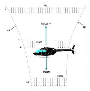
Figure a1: Flow model used for momentum theory analysis of a rotor in axial flight.
