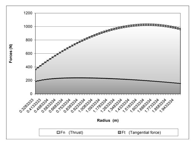
Figure b8: Thrust and tangential force repartitions on the blade
