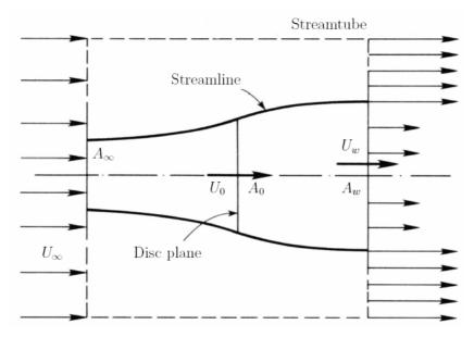
figure b1: Flow pattern inside the streamtube.
