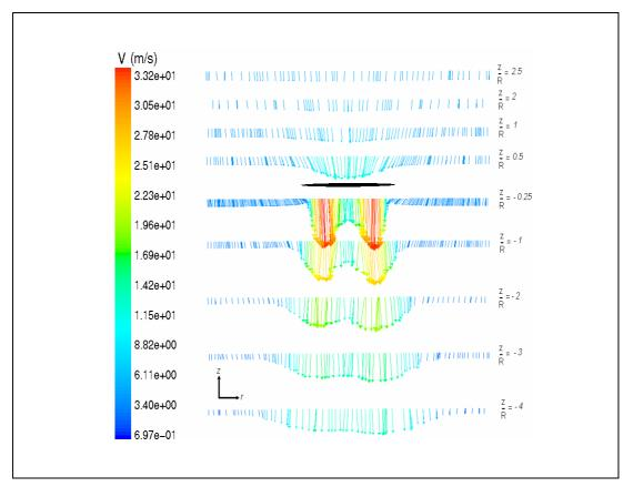
Figure a10: Velocity vectors (on the lines) coloured by Velocity magnitude
