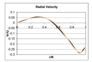
Figure a2: Radial velocity profile as function of the radial coordinates r normalised on the rotor.
