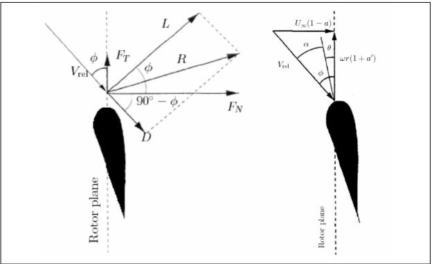
Figure b3: The local forces and velocity components on the blade
