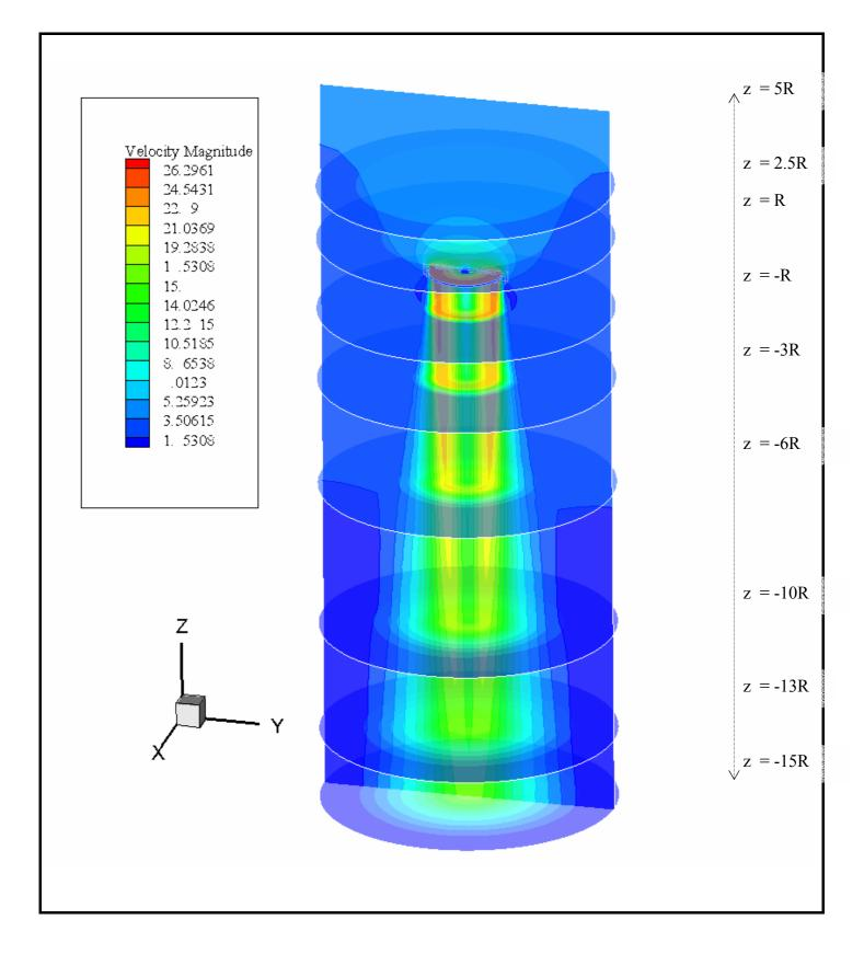
Figure b13: 3-Dimensional Contour Velocity Magnitude at different z coordinates
