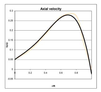
Figure a4: Axial velocity profile as function of the radial coordinates **r** normalised on the rotor.
