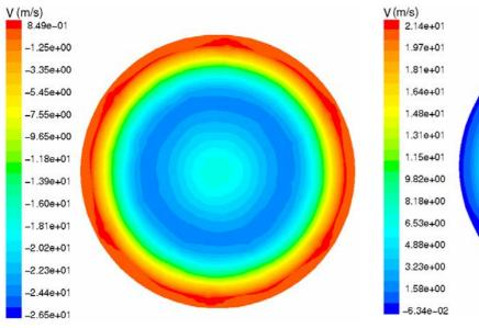
figure c7: Contour of axial velocity on the rotor
