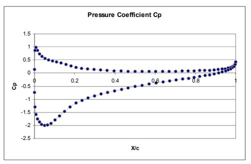
Figure b5: Pressure coefficient on the blade
