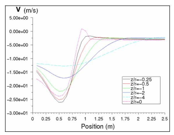
Figure a18: axial velocity profiles below the rotor as function of the radial coordinates r normalised
