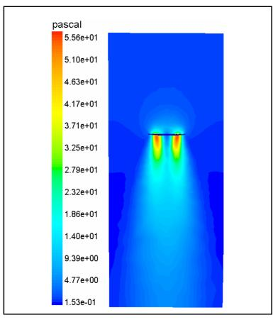
Figure a9: Contour of Dynamic Pressure on a plane
