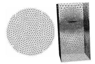
Figure a6 : triangular meshes on the rotor and tetrahedral meshes in the domain.
