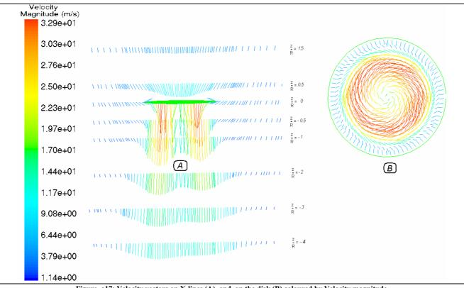
Figure a17: Velocity vectors on X-lines (A) and on the disk (B) coloured by Velocity magnitude
