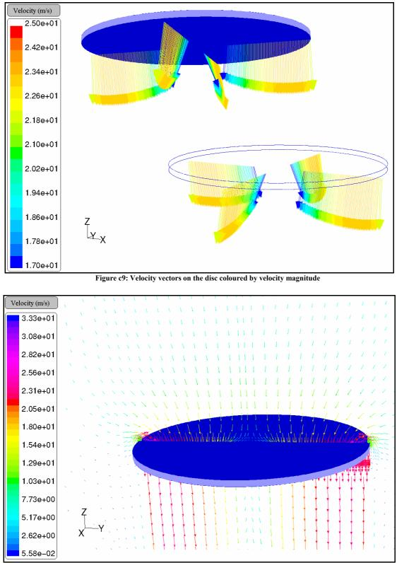
Figure c10: Velocity vectors on a plane coloured by velocity magnitude
