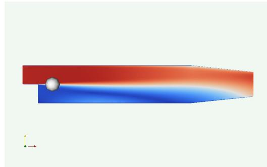
disc of injection of particles, velocity at t=1000
