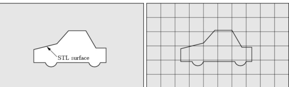
Aspect ratio should be around 1, with more than one cell in the z direction
