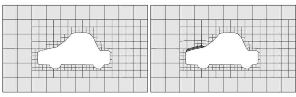
•After deleting the cells in the region specified, the points are snapped on the surface and spread depending on different parameters that one can find in snappyHexMeshDict
