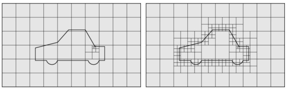
It starts according to a first edge specified in snappyHexMeshDict by the user. This edge must be inside the region to be meshed and must no coincide with a cell face either or before the refinement
