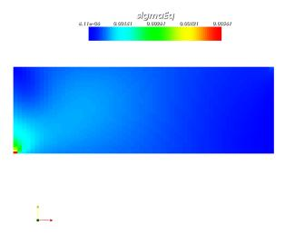
Figure 5: Magnitude of the stress tensor of the solid domain.
