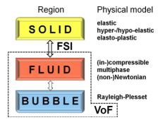
Fig. 1: Structure of the interaction model
