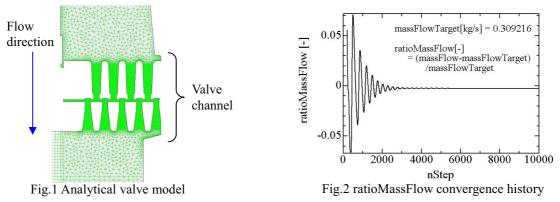
Key words: Valve, Optimization, Robustness, Taguchi method, Pressure loss, OpenFOAM, Target mass flow
