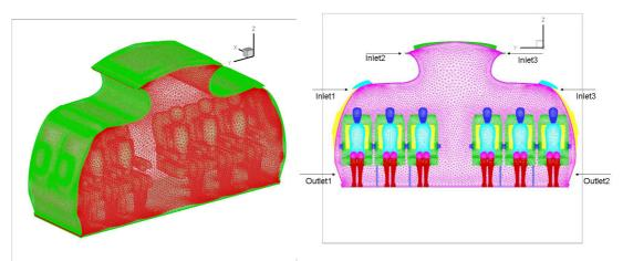
Fig 1.: Volume Mesh of a segment of an A-320 Fig. 2: SurfaceMesh of a A-320 cabin segment model cabin model
