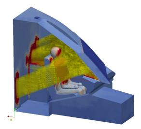
Figure 1: Iso-surfaces of solar radiation intensity and contours of wall temperature for an aircraft cockpit
