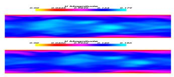
Fig.3 Qualitative effect of air particles in near wall region (up: w/o particle effects, Down: with particle effects)
